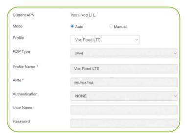
Save the new profile as the default and then proceed with the SIM activation steps as per page 1 of this guide. Please note that the images provided are of the ZTE MF286C router. Other router models may differ.
